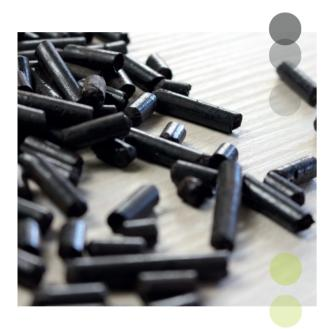
IBCs are formed when biomass is processed to energetically denser, storable and transportable intermediary products analogous to coal, oil and gaseous fossil energy carriers. They can be used directly for heat or power generation or further refined to final bioenergy or bio-based products. IBCs contribute to energy security, reduce greenhouse gas emissions and provide a sustainable alternative to fossil fuels in Europe.
